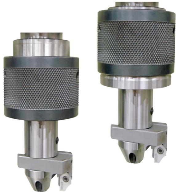
Rottler Patented exclusive multi-angle seat tooling eliminates the need for bounce springs. The Rottler patented tooling holds the ball driver firmly yet allows ball to float during seat cutting. This eliminates the cumbersome/ troublesome bounce springs but gives you the ultimate in valve seat concentricity.
