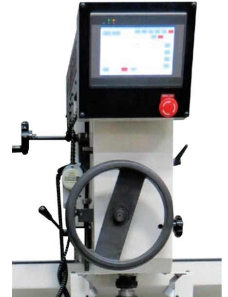
Rottler's trade mark that ensures that you our customer get the most accurate and versatile machine possible. Rottler combines precision carbide centering pilots with our light weight air float work head to give you perfect centering with the valve guide. This guarantees the best CONCENT of valve seat to valve guide centerline in the industry. Accuracy of .0005" per inch (.01mm per 25mm) is easily obtainable.
