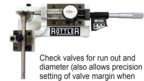
Check valves for run out and diameter (also allows precision setting of valve margin when setting up multi-angle cutters)
