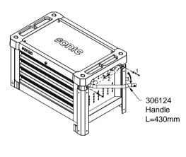
**3.** Position the handle on the topbox from left to right, tighten the screw securely.
