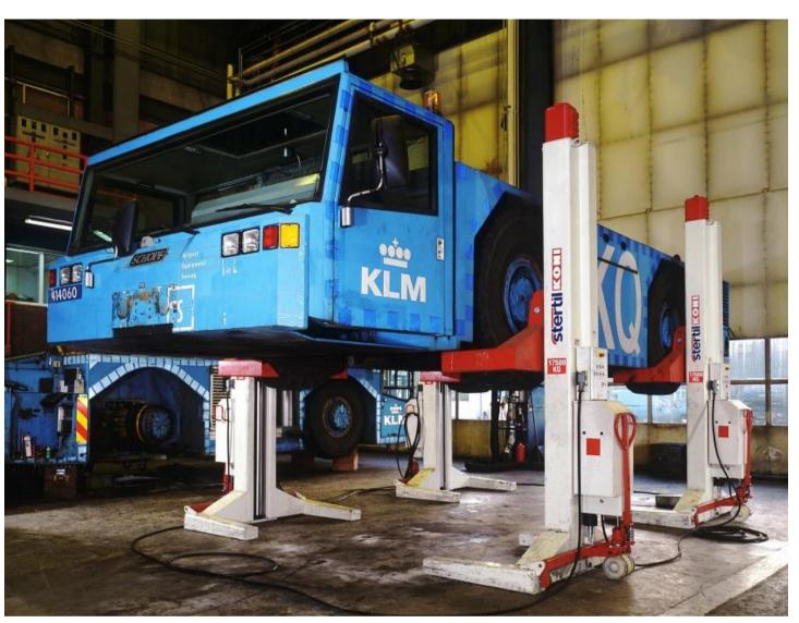
The flagship of our program is the mobile column lift, which is available with lifting capacity from 12,000 lbs. / 5.500 kg. up to 40,000 lbs. / 17.500 kg. per column. The advanced Stertil-Koni mobile column lift has earned its popularity because it has cleared the way for efficient and flexible workshop management.
