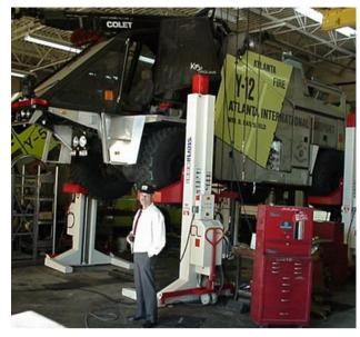
lifting columns in the world. The lifting height is over 2 metres, therefore it is comfortable to work with, even for tall people.
