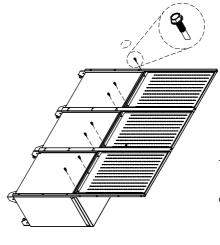
7.INSTALL CUPBOARD screws(M6X16) provided. Tighten securely. Hang the cupboards onto the screws and attach with the HEX socket head cap
