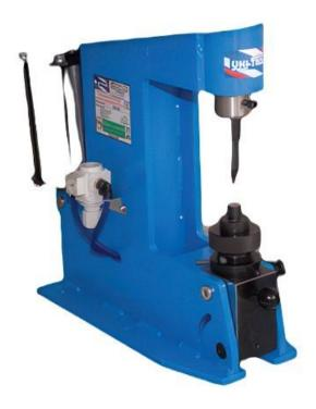
The PUN-1 device is intended for riveting brake linings used in motor vehicles with tubular/steel, brass, copper or solid aluminum rivets. The source of drive in the device is a pneumatic actuator controlled by a pedal.
